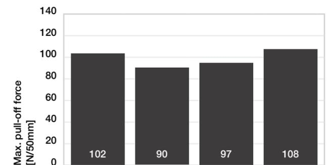
180° pull-off test after various exposure conditions
