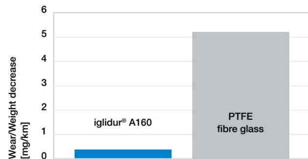
Linear wear against stainless steel pin (AISI 303)
