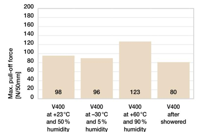
180° pull-off test after various exposure conditions
