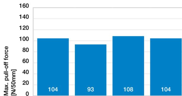
180° pull-off test after various exposure conditions
