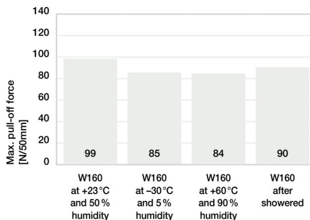
180° pull-off test after various exposure conditions
