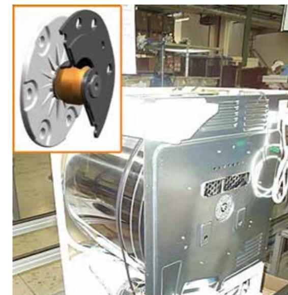
Drum bearing in a tumble dryer
