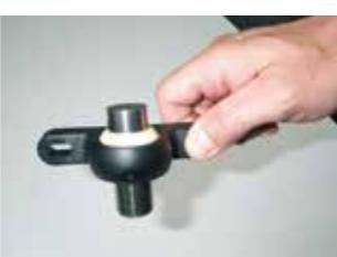
Tolerance test with plug gauge
